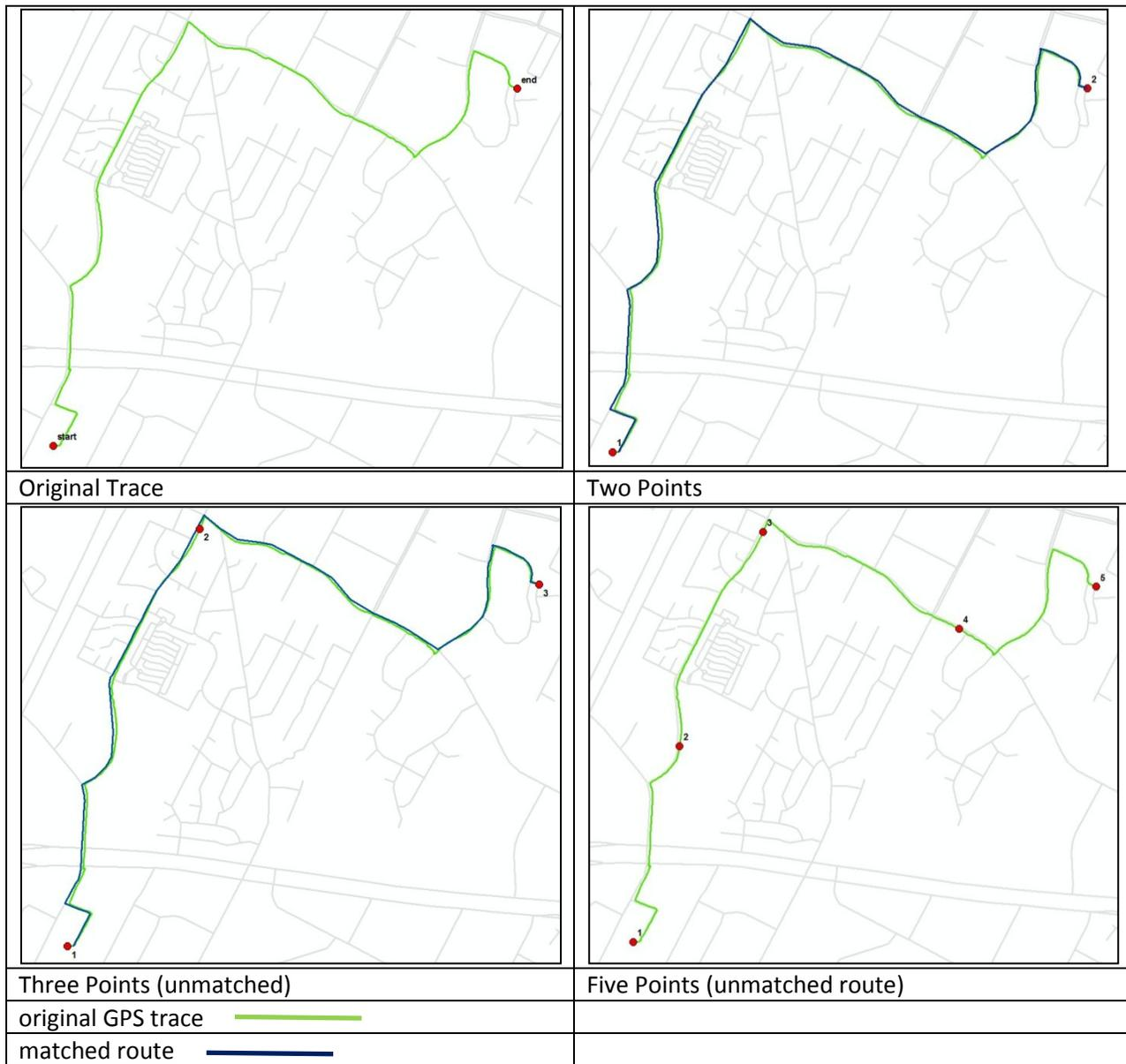
**Figure 42. Another Example of How Adding Points Results in Unmatched Routes**
