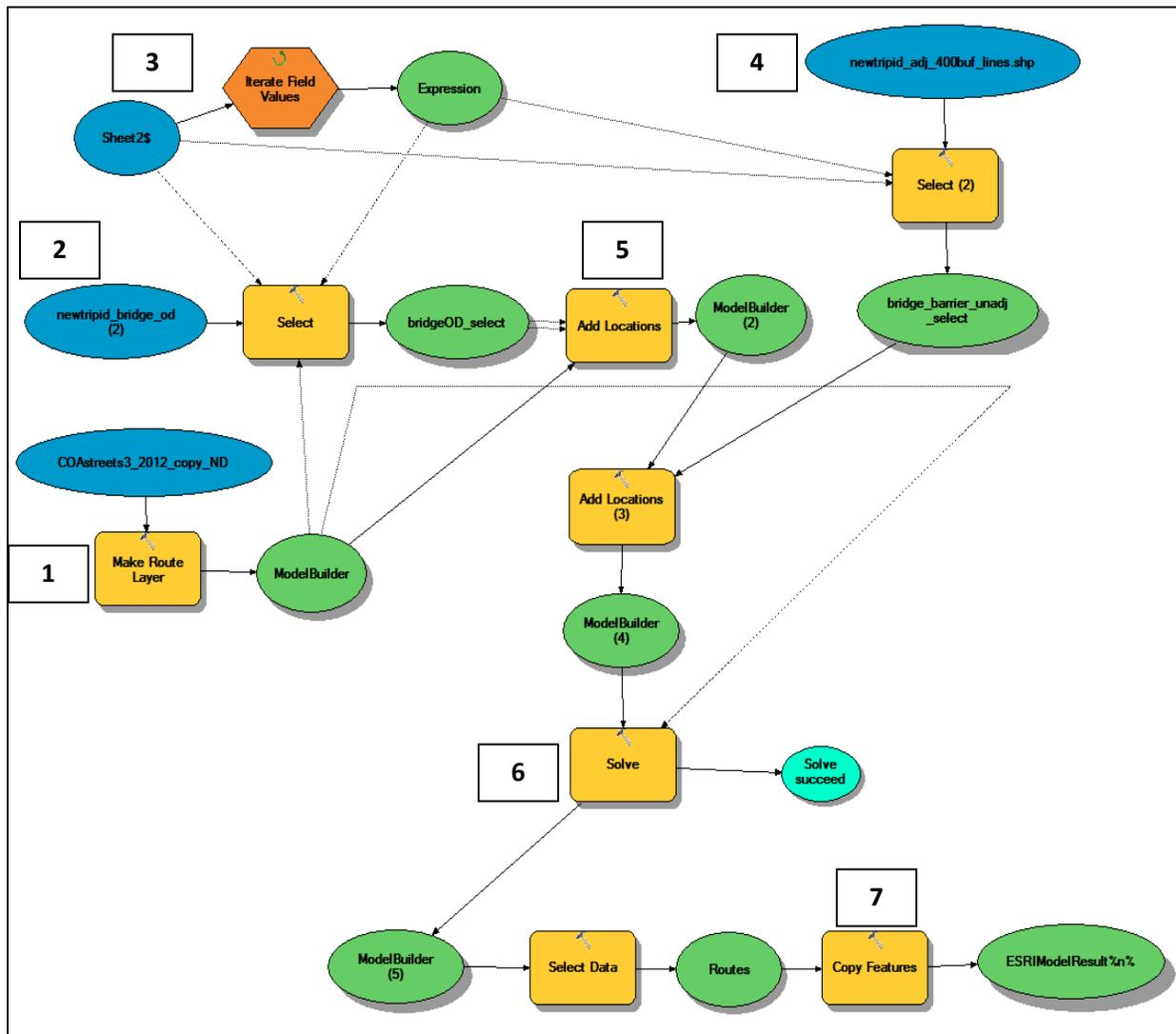
Figure 39. Model for Dalumpines and Scott (2011) Algorithm
